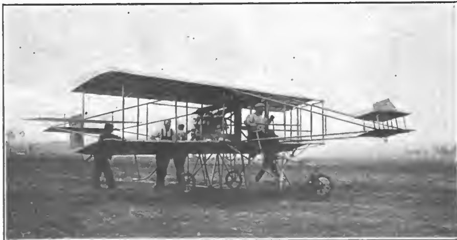
A Curtiss machine in which the allerons have been moved back of main planes and with single elevating rudder
